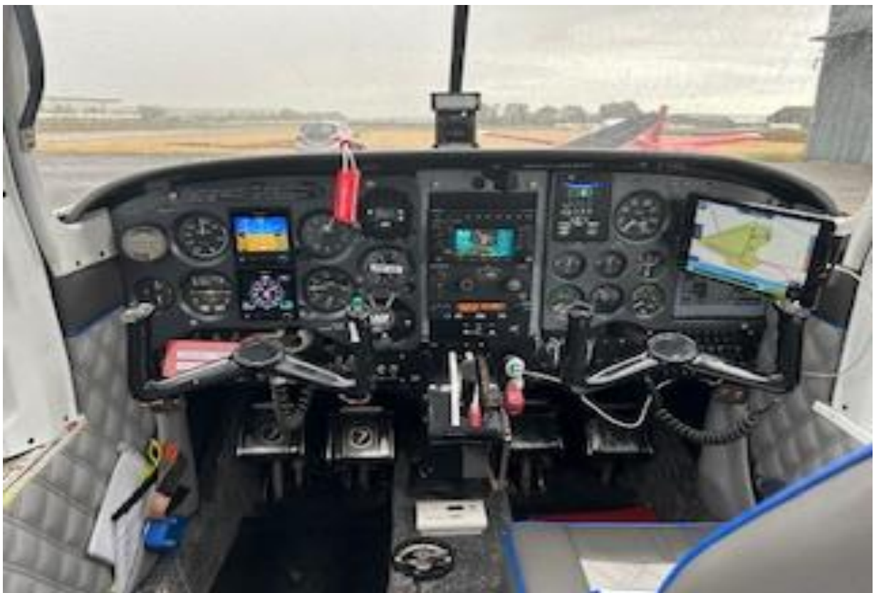
The IFR Instrument Panel and Upholstery GNS430 (Nav/Com; GPS/VOR/ILS; Com 1); Trig radio (Com 2); Two Garmin G5s; Trig Mode S Transponder; JPS engine monitor. iPad, with SkyDemon. Traffic alerting by Pilot Aware Rosetta unit (not shown).
