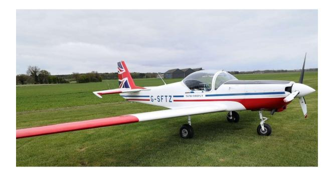
Tango Zulu is a two seat Slingsby Firefly T67M with a 160 hp fuel-injected Lycoming AEIO320 engine and three-blade constant-speed propeller. The fuel-injected engine with inverted fuel and oil systems allows the aircraft to perform aerobatics. A new 3 blade MT-propeller was installed in 2020 improving performance.
